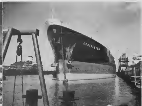
BOW LINE out, the Agri-gentium eases into No. 2 Finger Pier south. A spring line runs aft to a bollard to help slow down the vessel. CU CABUYA di mara afor, Agri-gentium ta slip den No. 2 Finger Pier. Un otro cabuya patras na e cabez di mara ta pa yuda wante e bapor.
